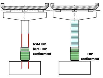
Furthermore, as shown in Figure 10, application of bond-based near-surface mounted (NSM) retrofitting technique using FRP bars was proposed and experimentally evaluated by Fahmy and Wu (2012, 2016).
