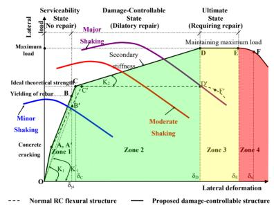
Figure 9 Idealised load-deformation behaviour of the proposed FRP-steel damage controlled structures (see online version for colours)
